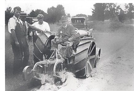
A Two-Bottom Plow that is Attached Directly to and Becomes a Unit with the Tractor. Harry Ferguson, of Belfast, Ireland, the inventor of the plow is shown on the tractor seat.
